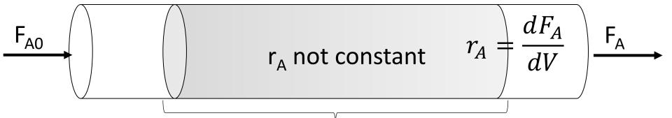
Changing conditions moving down reactor Tougher to model/extract rate parameters
